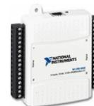
Figure 4.3 - NI DAQ USB 6009
